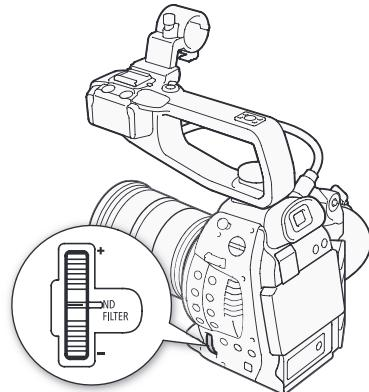
Turn the ND FILTER dial toward the + or - direction to select the desired ND filter setting.
