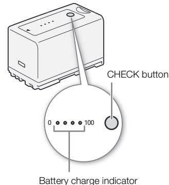
Press the BATT. INFO button to display the approximate remaining battery charge for about 5 seconds. Depending on the battery life, the battery information may not be displayed.
