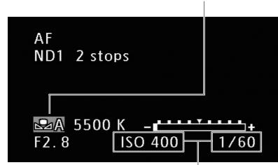
Push the joystick (◀▶) to highlight the ISO/Gain value or the Shutter value
