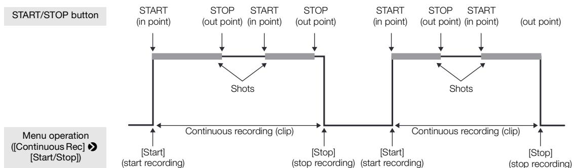
1 Open the continuous recording [Mode] submenu.
