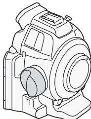
Minimal configuration with thumb rest. You will not be able to use the joystick, but you can set the joystick's functions (up/down/left/right/SET) to assignable buttons (☞ 91) to be able to change settings that require the joystick\*. Also, the control dial (☞ 60, 62) and MAGN. button/Assignable button 7 (☞ 91) cannot be used to operate the camcorder.
