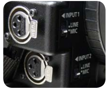
Two switches on front of camera
