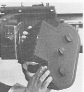
Figure 2b. Removing camera from stand.
